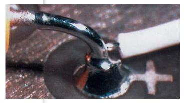
Wire contour or end is discernible in the solder connection.
