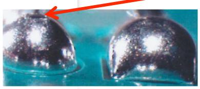
Lead not discernible due to excess solder, but is it visible on the left hand solder joint.
