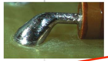
Solder in the bend radius is not cause for rejection provided the lead is properly formed and the topside bend radius is discernible.
