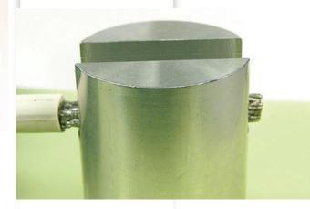
Lead or wire extends completely through slot and is discernible on the exit side.
