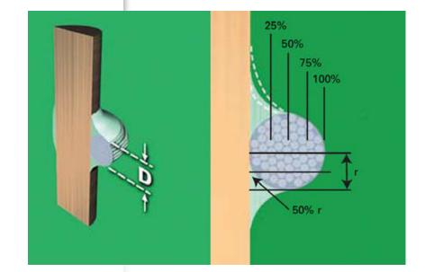
Solder wets the wire/lead and terminal and forms a discernible fillet feathering out to a smooth edge.
