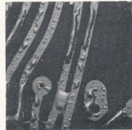
Fig. 17 Typical appearance of dewetted solder film on copper tracks of a printed circuit cleaned with an abrasive medium.
