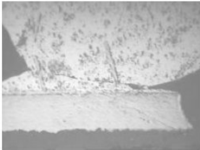
Figure 5. Solder joints made by 208°C peak/60-90TAL ramp profile.
